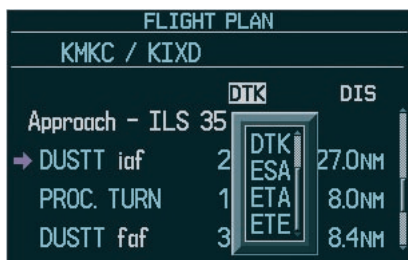
Figure 3.6.24 Change Fields on Flight Plan
