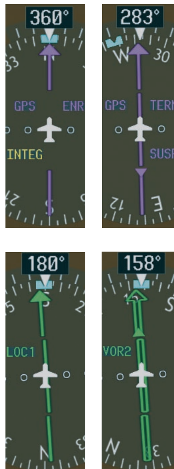
Figure 3.4.26 GPS INTEG, GPS SUSP, LOC1 and VOR2
