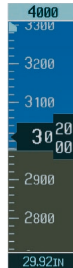
Figure 3.4.8 Altimeter within 1,000 ft of Reference Altitude
