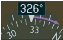
Figure 3.4.17 Turn Rate Indicator and Trend Vector
