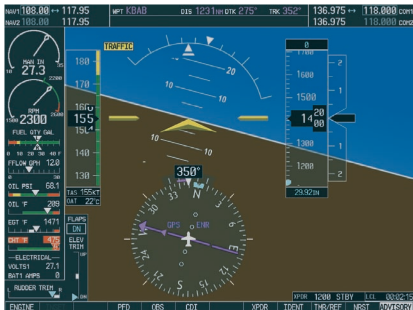
Figure 3.7.1 PFD Reversionary Mode
