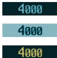
Figure 3.4.7 Colors Associated with the Altitude Alerter
